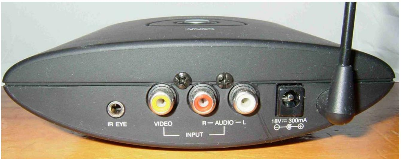
You will see on the back panel that there is an “IR EYE” socket (more later) plus the video and audio ‘Yellow, Red, White’ phono sockets. A lead is supplied which has the usual Yellow, Red, White phono plugs at one end and a SCART at the other.
