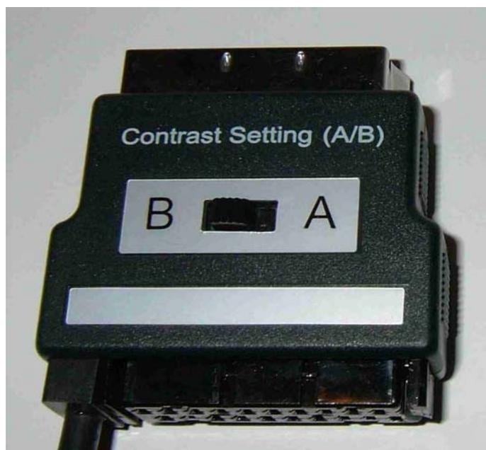
A switched attenuator is included as part of the SCART socket so that, if the signal from the DVD or Sky box is too great then it can be changed with the “A/B” switch.
