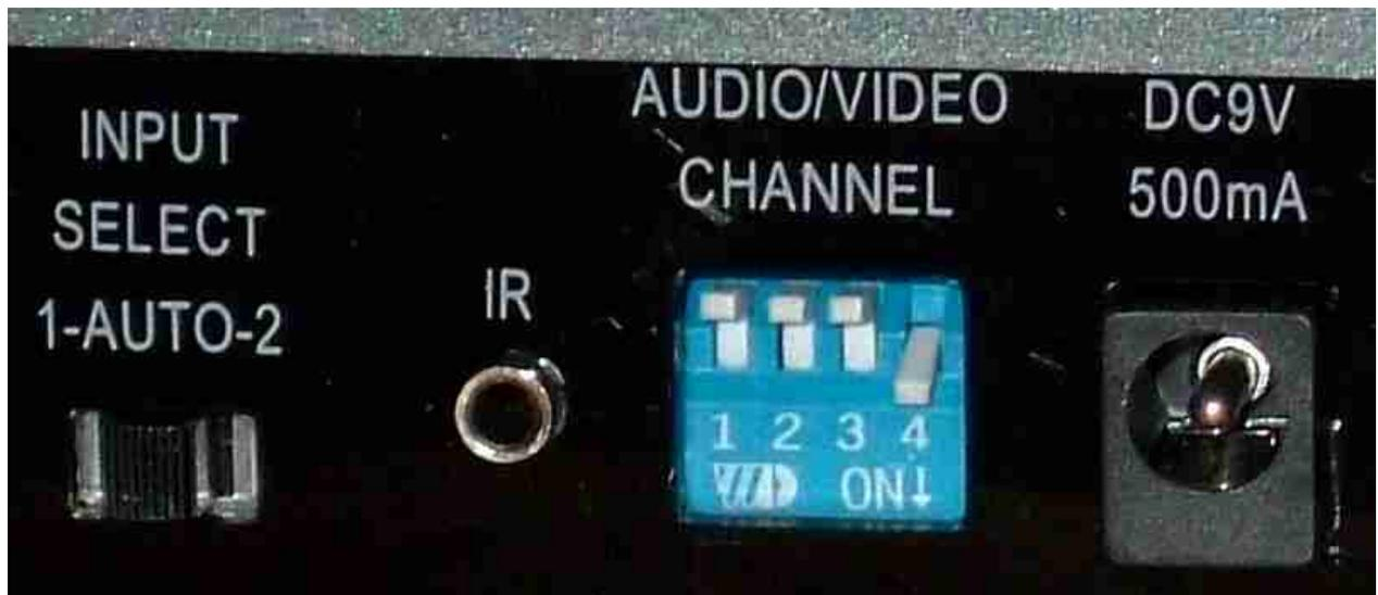
There are four channels available in the 2.4GHz band for this system. They are: 2.414GHz, 2.432GHz, 2.450GHz and 2.468GHz. The switches which you see in the photograph labelled "AUDIO/VIDEO CHANNEL" can be used to select any one of these four channels.
