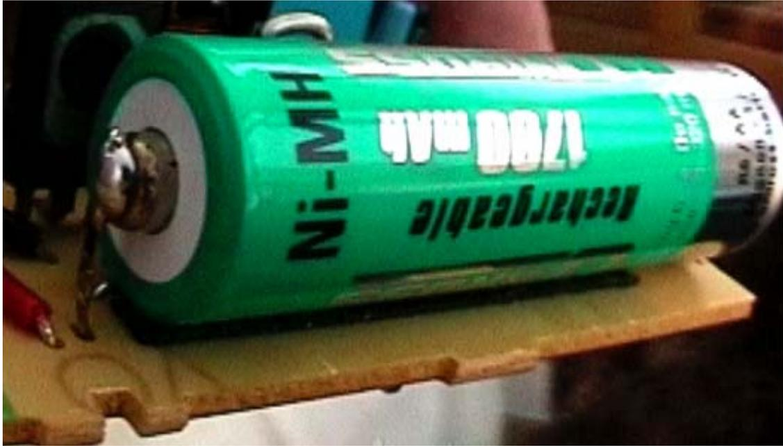
I use thin multi stranded flexible wire for the cell connections. I cut a length in excess of that which I need and thoroughly tin it with solder. I have found that the best way of making a good firm connection to the rechargeable cell is with a 'big' soldering iron but good results can be achieved with something smaller. A lot of heat for a short time is the key to success.
