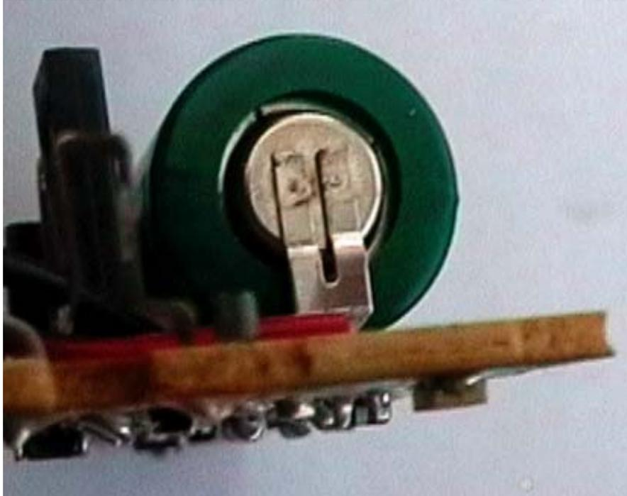
Usually batteries in dedicated equipment of this era are soldered in place. I have noticed that in more recent equipment such as portable CD players and chordless 'phones there is a tendency to make the rechargeable cells as easy to replace as a standard battery but, in older equipment, they are soldered in place.
